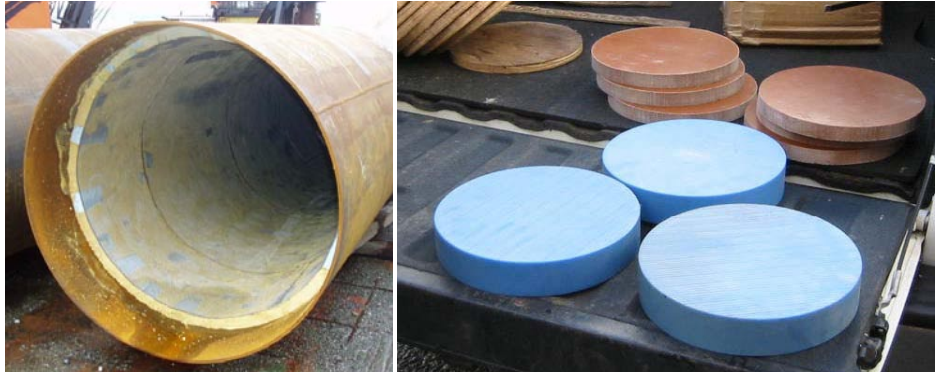
Figure 8 Left: circular steel casing with internal foam lining (Laughlin 2007). Right: wooden, micarta, and nylon pile caps at left, right, and bottom, respectively (Laughlin 2006)
