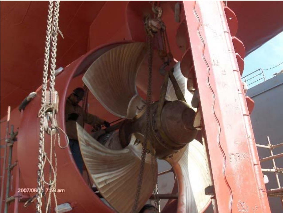
Figure 7 Forward skew propeller with sharp tip called “bird beak” (Spence et al. 2007)
